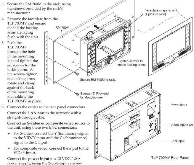
7. If you do not plan to calibrate the TLP 700MV immediately (see the TLP 700MV user's manual), replace the faceplate by pressing the catches on the faceplate into the corresponding holes on the sides of the panel.
